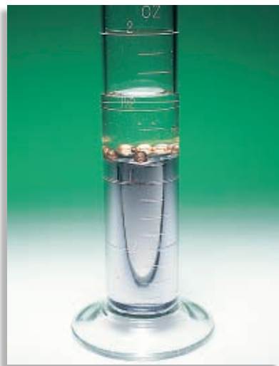
FIGURE 7 Density is the ratio of mass to volume. Both water and copper shot float on mercury because mercury is more dense.
