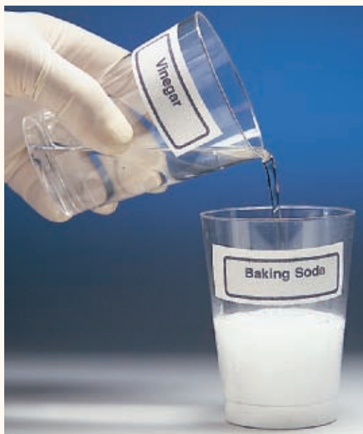
FIGURE A Slowly add the vinegar to prevent the reaction from getting out of control.
