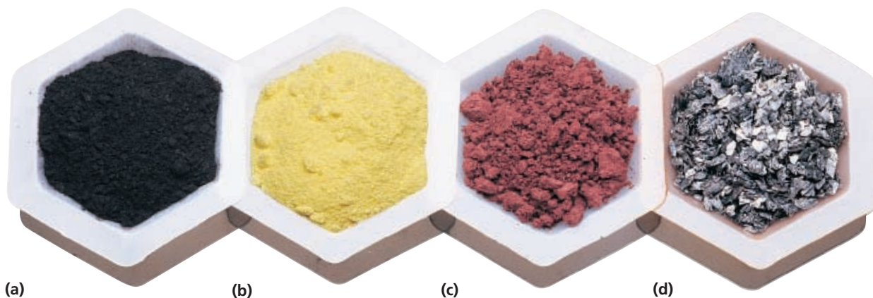
FIGURE 14 Various nonmetallic elements: (a) carbon, (b) sulfur, (c) phosphorus, and (d) iodine
