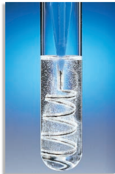
FIGURE 11 In this single-displacement reaction, the hydrogen in hydrochloric acid, \text{HCl} , is replaced by magnesium, \text{Mg} .
