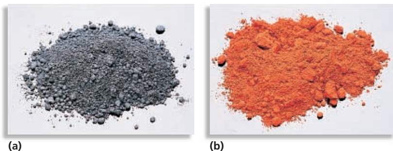
FIGURE 8 Iron, Fe, and oxygen, O_2 , combine to form two different oxides: (a) iron(II) oxide, FeO , and (b) iron(III) oxide, Fe_2O_3 .
