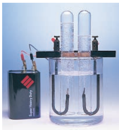
FIGURE 5 When an electric current is passed through water that has been made slightly conductive, the water molecules break down to yield hydrogen (in tube at right) and oxygen (in tube at left). Bubbles of each gas are evidence of the reaction. Note that twice as much hydrogen as oxygen is produced.
