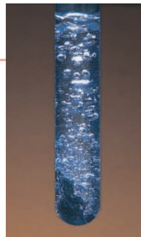
FIGURE 6 Solid zinc reacts with hydrochloric acid to form aqueous zinc chloride and hydrogen gas.
