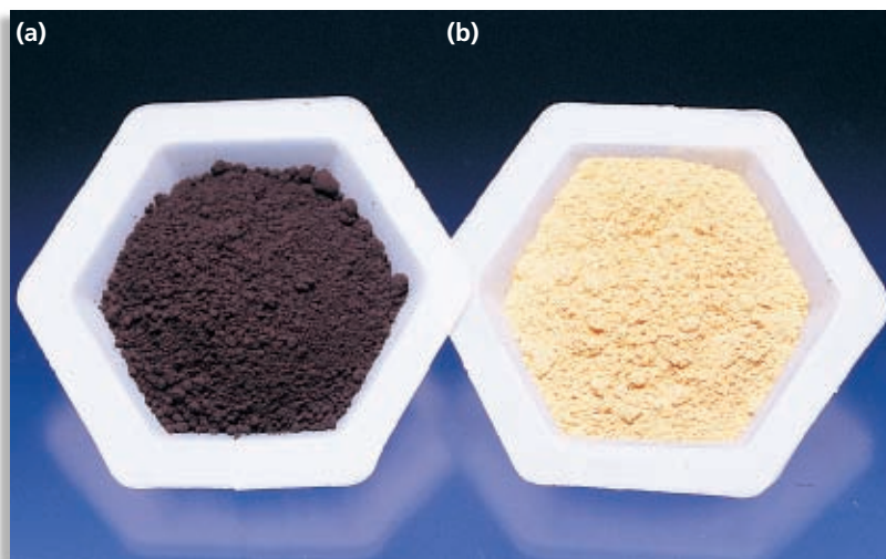
FIGURE 1 Different cations of the same metal form different compounds even when they combine with the same anion. Compare (a) lead(IV) oxide, \text{PbO}_2 , with (b) lead(II) oxide, \text{PbO} .
