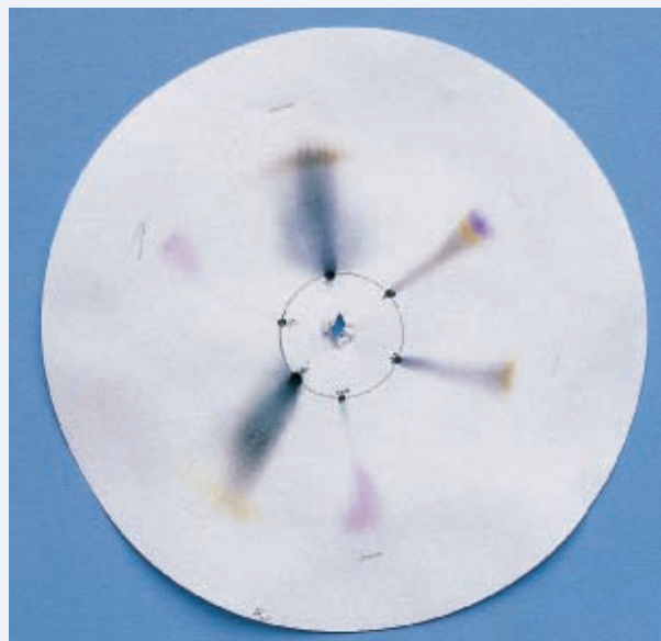
FIGURE E This chromatogram is unacceptable due to bleeding, or spread of the pigment front. Too much ink was used in the spot, or the ink was too soluble in the solvent.
