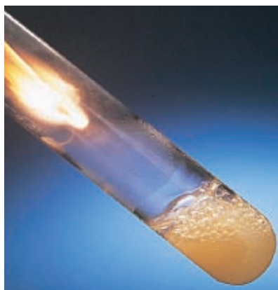
A glowing splint thrust into oxygen bursts into a bright flame.
