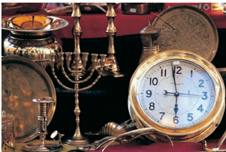
Brass has a high luster and resembles gold when cleaned and polished. A brass object can be coated with a varnish to prevent reactions of the alloy with air and water.
