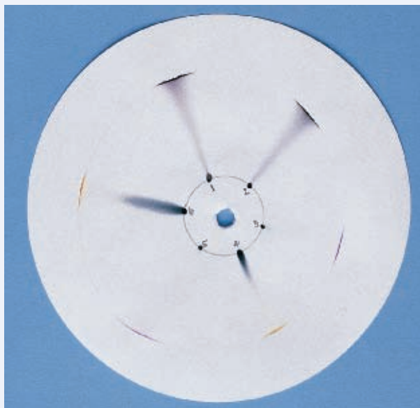
FIGURE D Each of the original spots has migrated along with the solvent toward the outer edge of the filter paper. For each substance that was a mixture, you should see more than one distinct spot of color in its trace.
