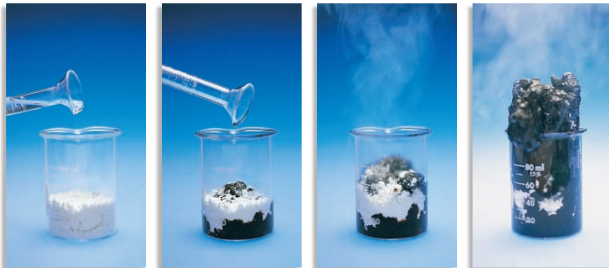
FIGURE 17 Sucrose is dehydrated when it reacts with concentrated sulfuric acid. Elimination of water produces a compound that is mostly carbon.
