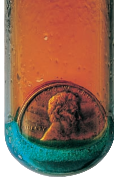
FIGURE 3 Copper is oxidized and nitrogen dioxide is produced when this penny is placed in a concentrated nitric acid solution.
