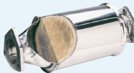
▲ The ceramic honeycomb inside a catalytic converter is coated with a metal catalyst.
