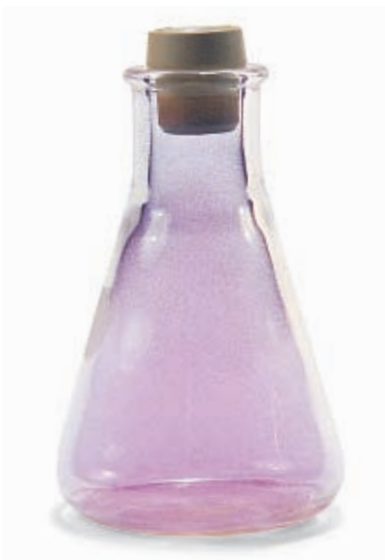
FIGURE 2 Colorless hydrogen iodide gas, HI, decomposes into colorless hydrogen gas and violet iodine gas. Some of the hydrogen gas and iodine gas will reform HI.
