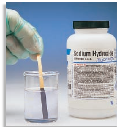
FIGURE 5 pH paper turns blue in the presence of this solution of sodium hydroxide.
