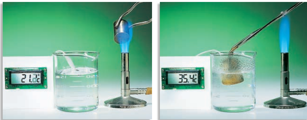
FIGURE 1 The direction of energy transfer is determined by the temperature differences between the objects within a system. The energy is transferred as heat from the hotter brass bar to the cooler water. This energy transfer will continue until the bar and the water reach the same temperature.
