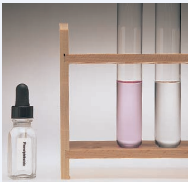
FIGURE A After adding phenolphthalein indicator, you can more easily determine which solution is acidic and which solution is basic.
