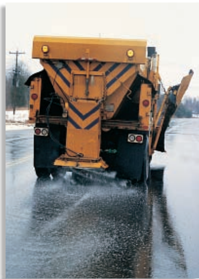
FIGURE 10 The salts applied to icy roads are electrolytes. They lower the freezing point of water and melt the ice.
